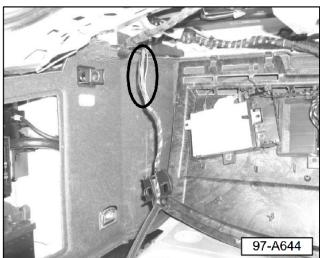
Splice in new trunk lid sectioned harness in location circled.
