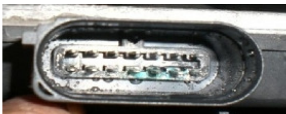
Illustration 12: corroded brake servo control unit contacts
