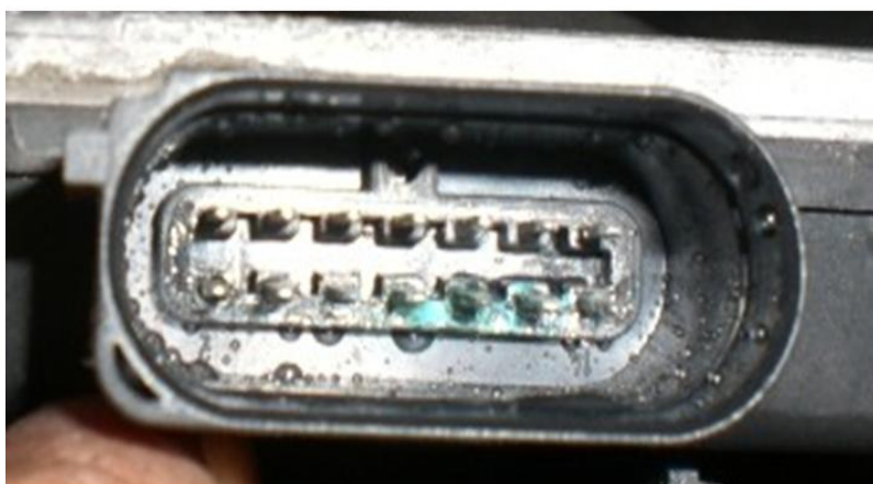
Illustration 18: corroded brake servo control unit contacts
