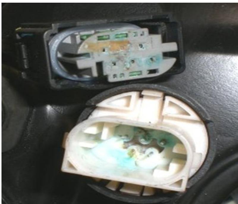
Illustration 13: corroded contacts on brake servo
