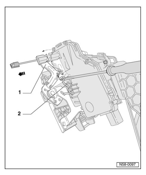
= Pull the operating lever - 1 - in the direction of the - arrow - .
