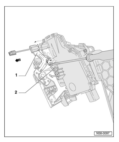
Using a screwdriver, tension the spring - 2 - secured to the door lock in the direction of the arrow and engage the lock lever in the spring.
