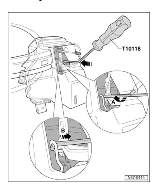
Guide the assembly tool T 10118 into the door through the opening in the inner door panel.
