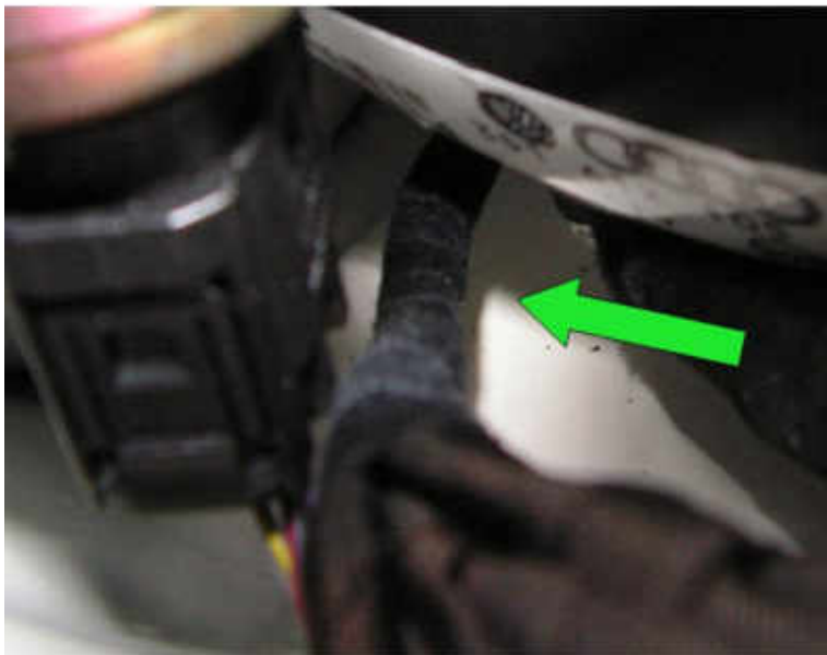
Illustration 10.1: Routing of the adapter wiring loom under brake servo
