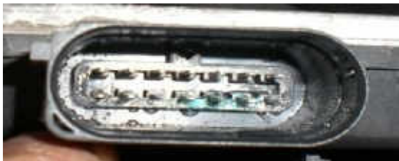
Illustration 12: corroded brake servo control unit contacts
