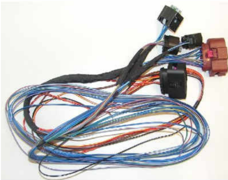
Illustration 4: Adapter wiring loom between brake servo control unit and brake servo
