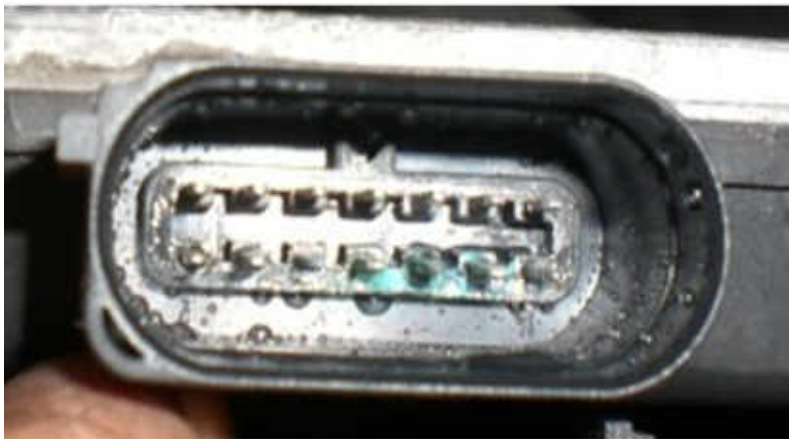
Illustration 18: corroded brake servo control unit contacts
