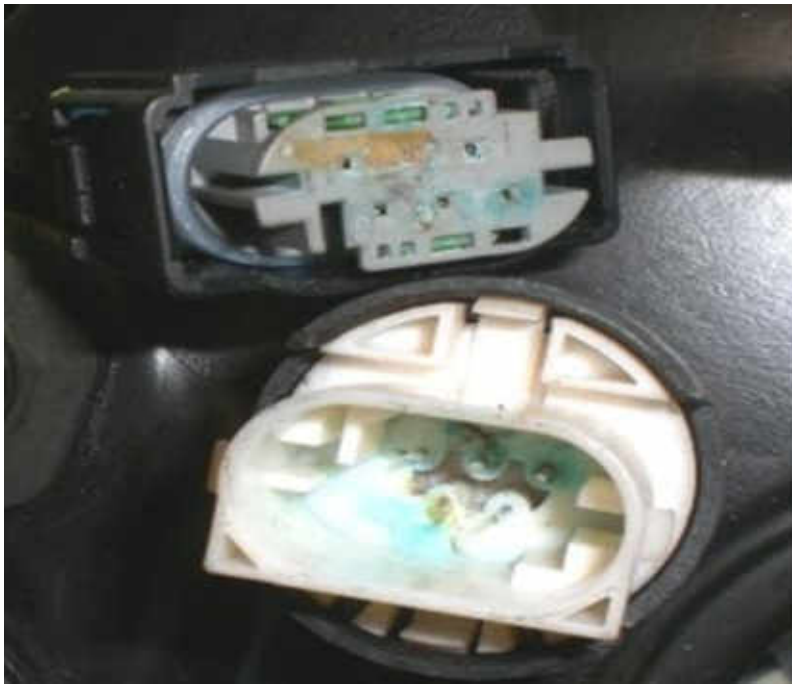
Illustration 13: corroded contacts on brake servo
