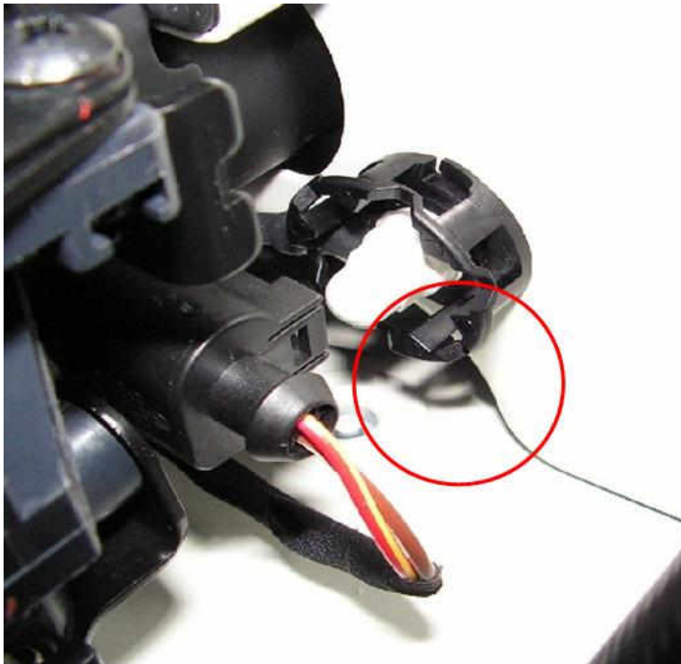
Illustration 9: Routing of the adapter wiring loom on the plenum chamber
