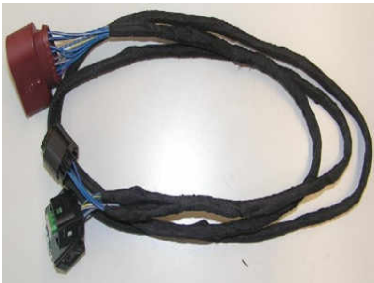
Illustration 8: Protection of adapter cable with tape
