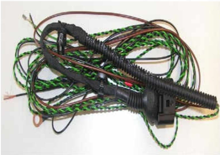
Illustration 3: Green/black cables twisted with earth connection
